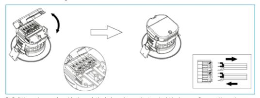
3) Pull the mains supply cable through the hole and open the terminal block cover. Connect the mains supply cable into the terminals ensuring that the correct polarity is observed. Close the terminal block cover tightly to secure the cable in place.
