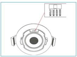
2) Prior to installation, the colour temperature of the LED light source must be selected for the desired application. The colour temperature selector switch is located on top of the driver housing. Three options are available. Warm White. Neutral White and Cool White.
