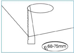
1) Select the required mounting position in the ceiling and cut out a circular hole 65mm in diameter. Do not exceed the cutting diameter and ensure that cut outs are spaced adequately to provide clearance from any joists, beams or cables within the ceiling void.
