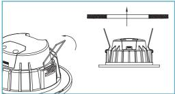
Hold back the spring clip and push the lamp in. Make sure the downlight is fixed securely and flush against the ceiling.
