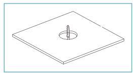
Cut a suitable hole in the ceiling as per the cut-out details. Ensure that it does not damage electrical cables, water/gas pipes or ceiling joists.
