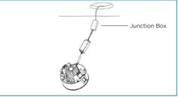
Connect the driver to the power and luminaire ensuring all wires are in the right location.
