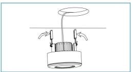
3) Hold back the spring clip and push the lamp in. Make sure the downlight is fixed securely and flush against the ceiling.
