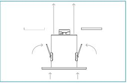
Push the spring clips upwards and insert downlight can into the ceiling hole previously cut-out. The clips will flip back and secure the can to the ceiling.
