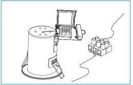
Connect the electrical supply cable, observing the correct polarity. (Live = Brown, Neutral = Blue)
