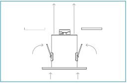
4) Push the spring clips upwards and insert downlight can into the ceiling hole previously cut-out. The clips will flip back and secure the can to the ceiling.
