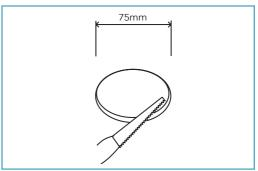
With a suitable mounting position identified, carefully cut-out the recommended size based on the model you are installing.
