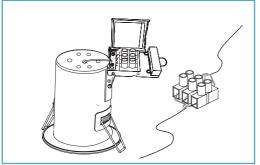
3) Connect the electrical supply cable, observing the correct polarity. (Live = Brown, Neutral = Blue)
