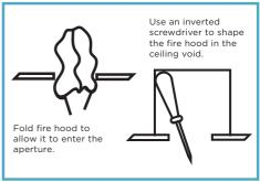
3) Secure the fire hood: Hold the fitting straps, align pins or tacks with the plasterboard and push through the hole and into the plasterboard. Any excess material on the straps can be removed or secured so that it will not intervene with the installation. Juminaire or performance.
