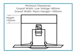
2) Whilst in the ceiling void, carefully shape the fire hood with an inverted screwdriver handle (or similar blunt object), push it up into the fire hood and move it around to completely open out the cover.
