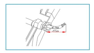
4) Bare conductor length: 8mm
