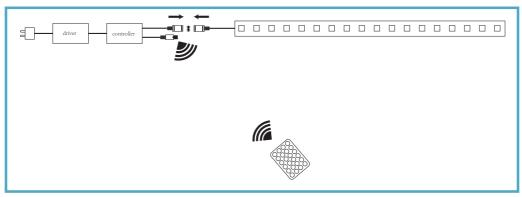
2) Connect the LED strip to the IR Controller by carefully inserting the 4 pin connector into each female input, aligning the arrows on each side. Connect the IR controller to an appropriate driver.
