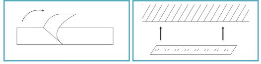
1) Peel the backing off all strips to reveal the adhesive coating. Carefully secure the strip to the surface in the required position.
