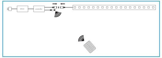
2) Connect the LED strip to the IR Controller by carefully inserting the 4 pin connector into each female input, aligning the arrows on each side. Connect the IR controller to an appropriate driver.
