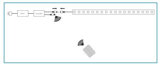
2) Connect the LED strip to the dimming controller. Connect the dimming controller to an appropriate driver.
