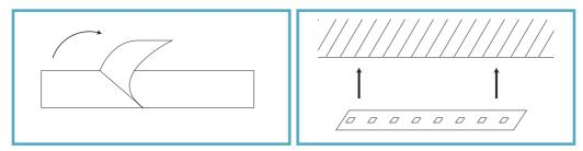
1) Peel the backing off all strips to reveal the adhesive coating. Carefully secure the strip to the surface in the required position.
