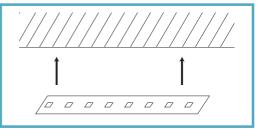
1) Peel the backing off all strips to reveal the adhesive coating. Carefully secure the strip to the surface in the required position.
