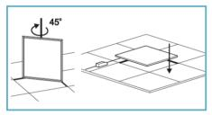
**3)** Install the panel into the ceiling by inserting at a 45° angle and moving to lay level and flat.
