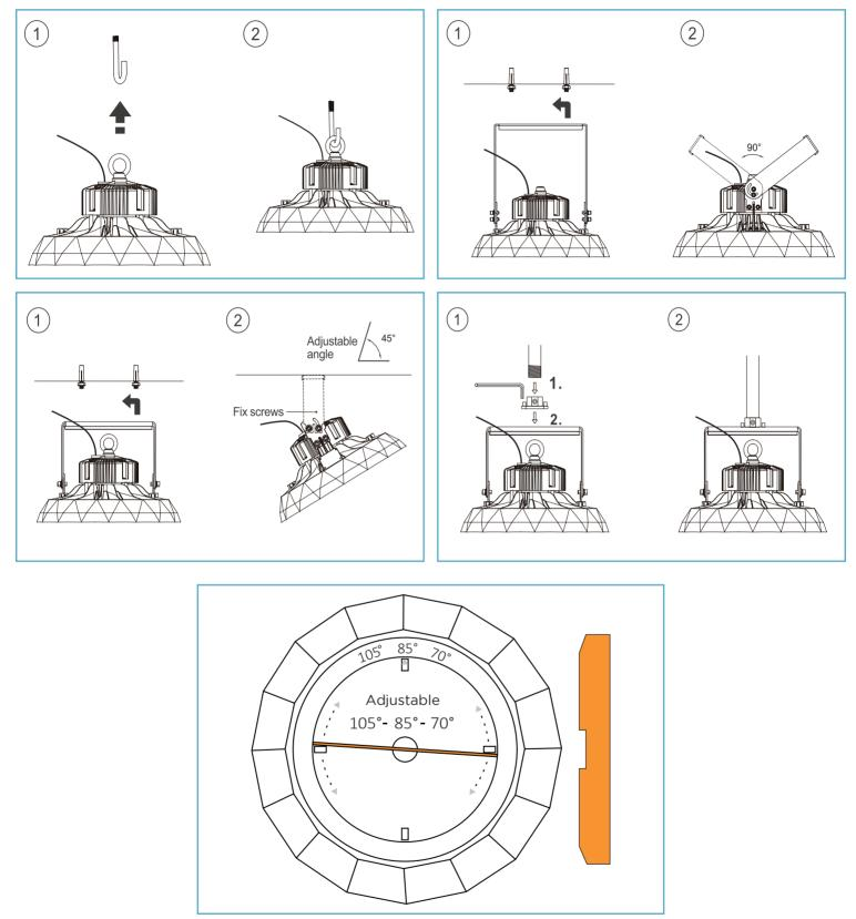
Use the provided tool to adjust the beam angle of the highbay.
