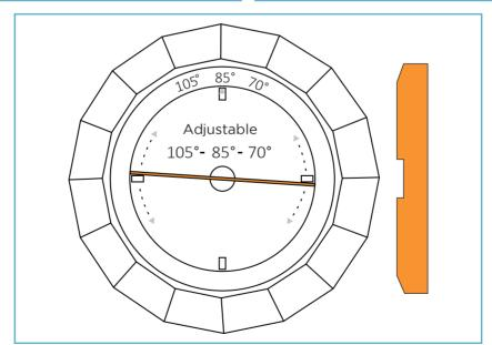
Use the provided tool to adjust the beam angle of the highbay.
