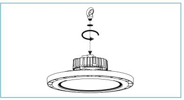
2) Attach enclosed mounting hook, ensuring you tighten to a torque setting of no less than 8.5 Nm.
