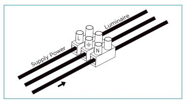
4) Connect mains power to the luminaire using a straight screwdriver to fix the wire into the right position. L to brown cable, N to blue cable, Green/Yellow as earth cable.
