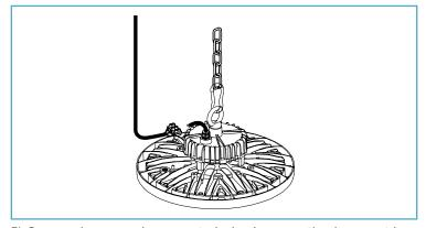
**5)** Once mains power is connected, check connection is correct by switching the power supply on.
