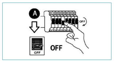
1) Ensure mains supply is switched off before installation.
