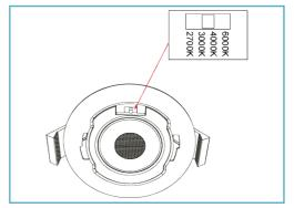
2) Prior to installation, the colour temperature of the LED light source must be selected for the desired application. The colour temperature selector switch is located on top of the driver housing. Three options are available. Warm White, Neutral White and Cool White.
