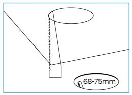
Select the required mounting position in the ceiling and cut out a circular hole 65mm in diameter. Do not exceed the cutting diameter and ensure that cut outs are spaced adequately to provide clearance from any joists, beams or cables within the ceiling void.
