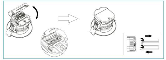
**3)** Pull the mains supply cable through the hole and open the terminal block cover. Connect the mains supply cable into the terminals ensuring that the correct polarity is observed. Close the terminal block cover tightly to secure the cable in place.
