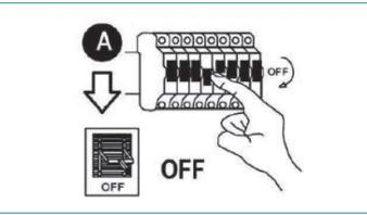
1) Ensure mains supply is switched off before installation.
