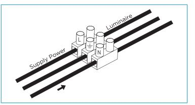
**4)** Connect mains power to the luminaire using a suitable IP rated connector.
