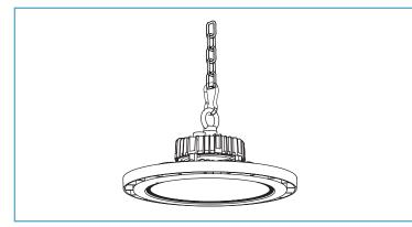
3) Check that mounting method is of suitable weight rating to support the luminaire safely. Allow additional length within mounting if the designated location is affected by air movement, which could cause the luminaire to swing or rotate.
