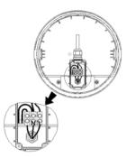
4 • Insert and connect the power cable.
